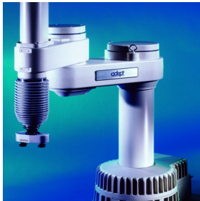
The Adept One SCARA robot (Debuted 1984).
