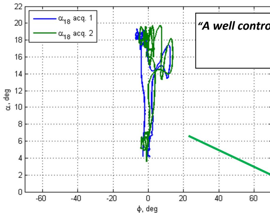
*"A well controllable aircraft during stall and post-stall flight"*
