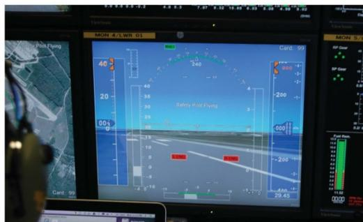
The research pilot station has standard displays with synthetic vision the primary view
