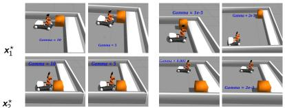
End pose of the KUKA platform with our iDG formulation given different goal states and  $\gamma$ -values.
