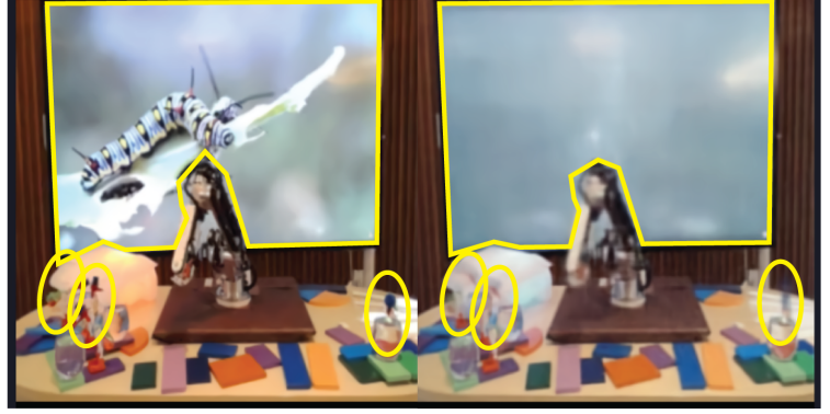
Figure 2: AC-State Successfully Removes Exogenous Noise: In our experiments, we demonstrate an application of AC-State in a Robot Learning Task. AC-State discovers the control-endogenous latent state in a visual robotic setting with temporally correlated distractors: a TV, flashing lights, and drinking bird toys (left). The reconstruction from AC-State decoder captures the arm’s position, while ignoring all the irrelevant background distractors (right). This latent representation captures the relevant parts of the world without any supervision, reward signal, or hard-coded assumptions.
